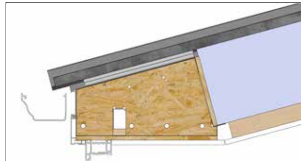
This image is the plaster line detail when at 15°
